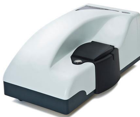
Figure 37 - Malvern® Zetasizer Nano ZS used in the DLS analyses (determine Z_{av} and PDI ).
