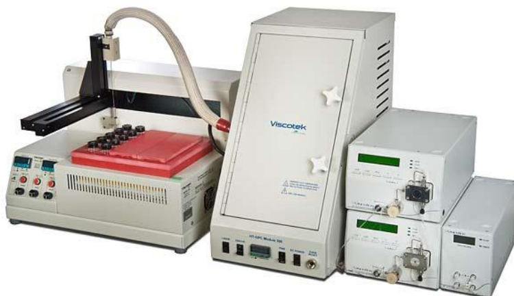
Figure 36- Viscotek Malvern® HT-GPC Module 350 A used to determine polymer molar masses and dispersities by SEC.
