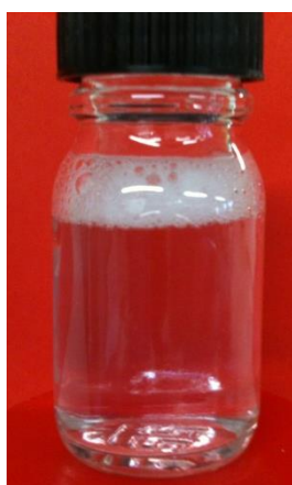
Figure 58 - Polymerization sample of FREPE (RL-PE 26) (1h, 100 bar, 50 mg AIBA, 0.3 g PEG-X, 250 rpm, T=70°C).
